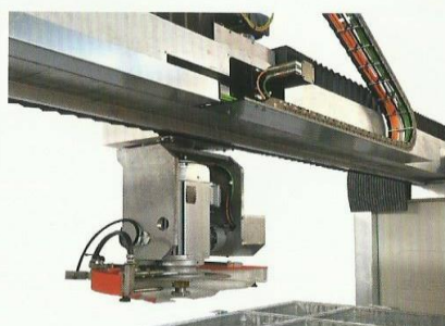
Disco inclinato a 90°. Disc inclined at 90°.
